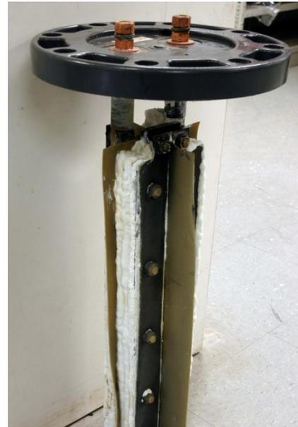
A cell stack with calcium bridged plates.
