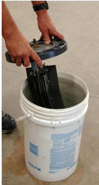
**Clean the cell when calcium buildup is present with the ChlorKing® Acid Wash System (non-reverse polarity system)**
