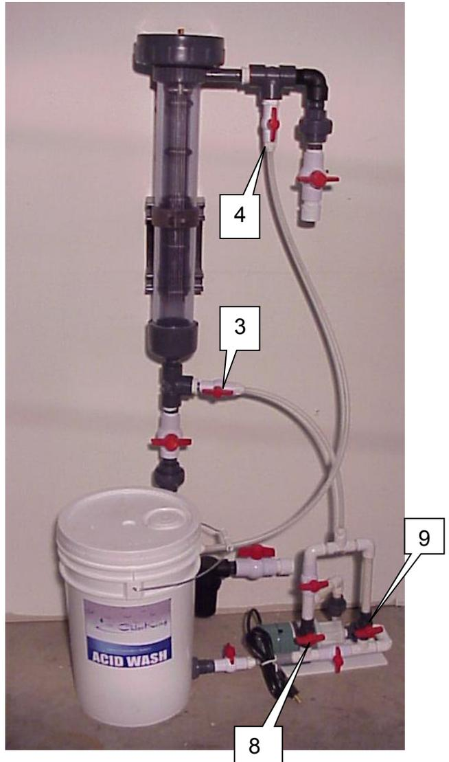
Plug the Acid Wash pump in to a 120 VAC source and start the wash cycle. Allow the pump to run until the cell is clean.
