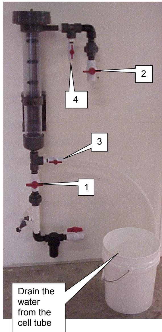
Connect the acid wash tank and pump to the acid wash valves [3] and [4] as shown in the photo on the right.
