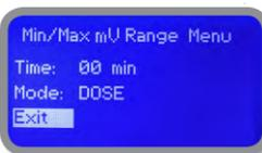
Time: How long the Hi/Lo number has to be reached before chemical dosing pumps stop dosing.
