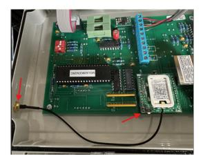
**Step 3: Install Ethernet Module**
