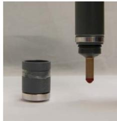
**Warning: The membrane may be damaged if the vent is not opened while removing the membrane cap.**
