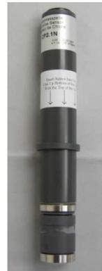
Slide the smaller diameter O-Ring up the sensor body until it rests against the Probe Ring.
