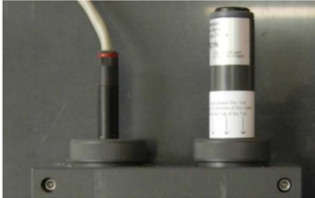
The voltage applied by the controller to the Free Chlorine Sensor polarizes the surface of the gold cathode. The polarization period (one hour) must elapse before calibration is performed based on the results acquired through the use of a DPD test kit.
