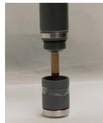
To re-install the sensor in the flow cell:
