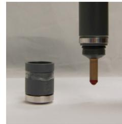
**Warning:** The membrane may be damaged if the vent is not opened while removing the membrane cap.
