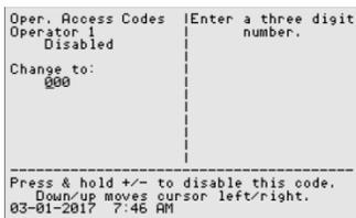
Pressing and holding the +/- button disables the access code, while pressing enter will enable and set the access code to the value on the screen.
